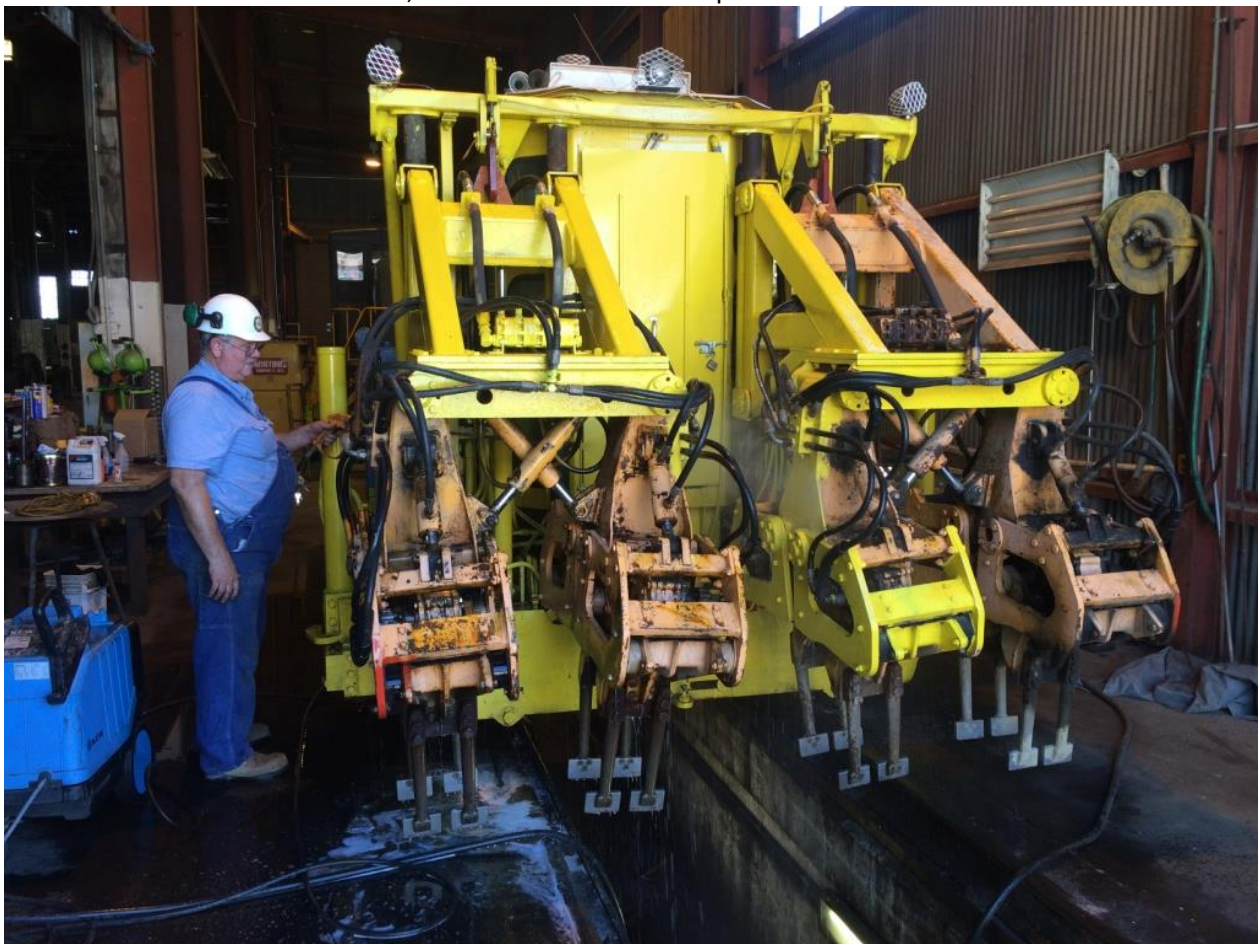
Time for a bath: Chris steam-cleans years of muck and grease off the work-heads
