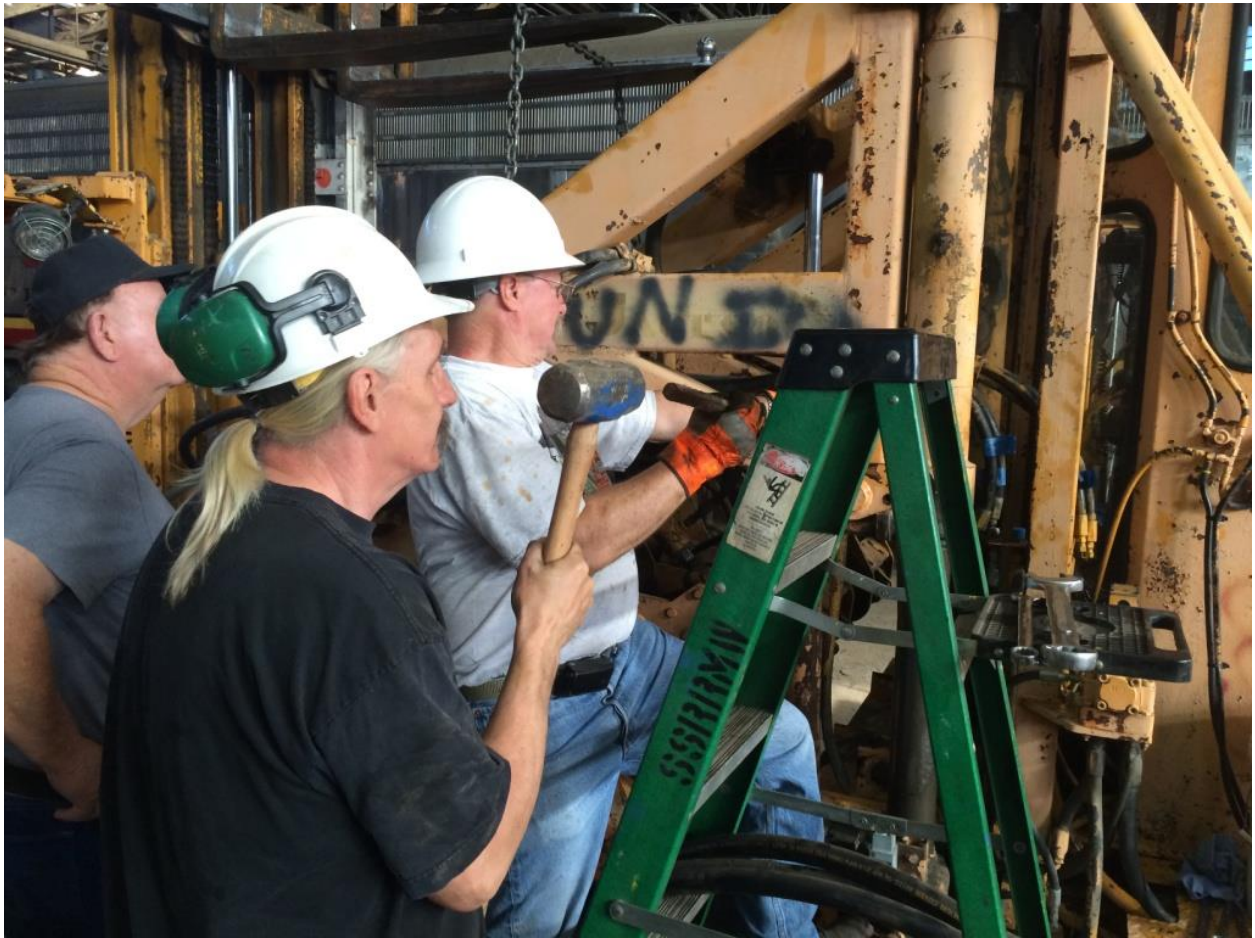
Fred and Mike pound out a pin holding the work-heads on to the old-old tamper
