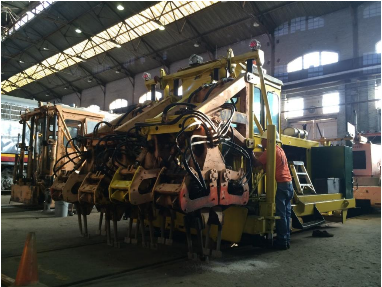
Both work-heads now installed on the new-old tamper
