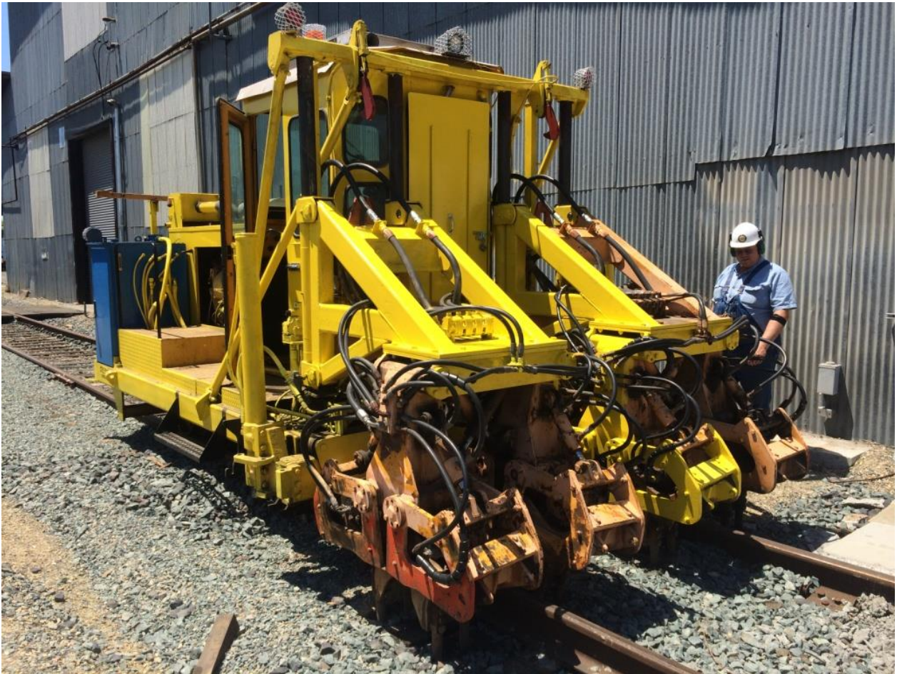
On builder's trials, the refitted new-old tamper is tested for the first time
